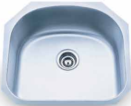
861 Stainless Steel (18 Gauge) Undermount Large Utility Sink. 304 SS with Satin Finish. Insulated Bottom. Overall Measurements: 23-1/4" x 20-7/8" x 9" Bowl Measurements: 21-1/4" x 18-7/8" x 9" Drain Opening: 3-1/2"
